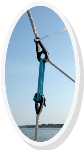
Shroud adjuster system using our stopper knot lashing to connect the lower shroud to the upper. See the website for more info on our stopper knot .
