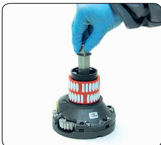
6. Slide out the central shaft n°18
