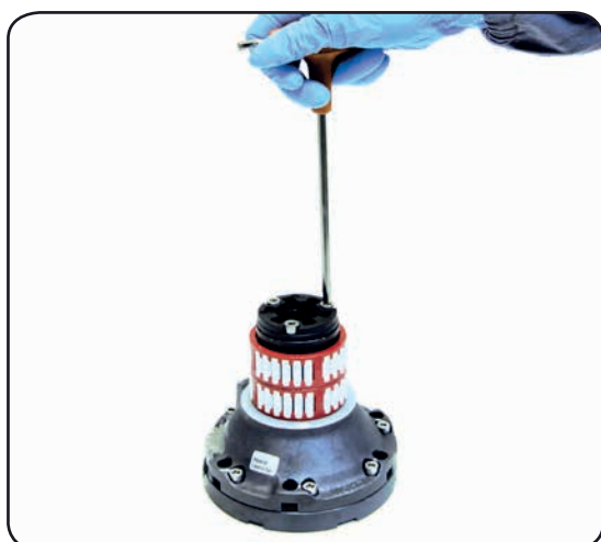
4. Completely unscrew the three screws n° 24
