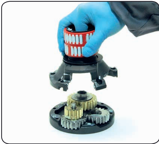
8. Remove the drum support n°14 Important: washer n°11 may remain inside the drum support!
