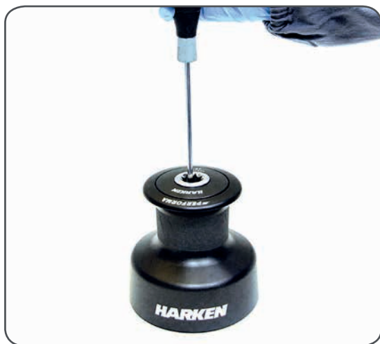
1. Unscrew the central screw (⚙️ 2Nm/18 in-lb)
