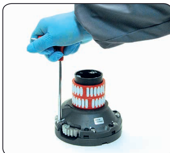
7. Unscrew the 6 hex screws n°15 ( \approx 8Nm/71 in-lb)
