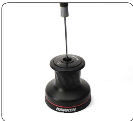
1. Unscrew the central screw (⚙️ 2Nm/18 in-lb)
