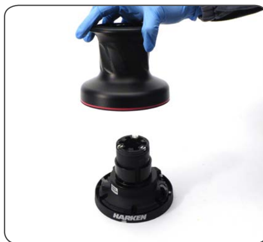
2. Lift off the drum n°13 with the socket n°18
