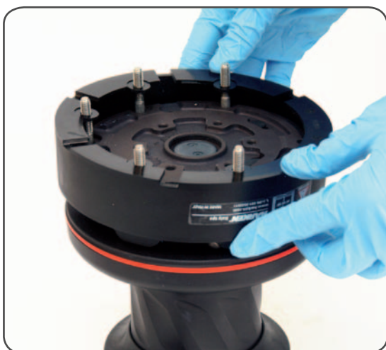
4. Reposition the skirt n°2 in its housing
