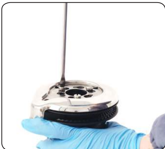
3. Unscrew the three screws n°18 ( \approx 4\text{Nm}/35\text{ in-lb} )
