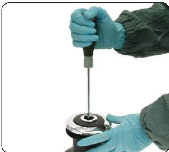
1. Unscrew the central screw ( \approx 2\text{Nm}/18\text{ in-lb} )
