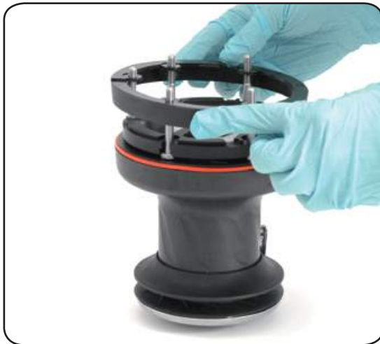
4. Reposition the skirt n°2 in its housing
