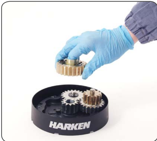
10. Remove the gearing n°7 and remove the pawls n°4. To facilitate the operation press the spring against the pawl with a blade.
