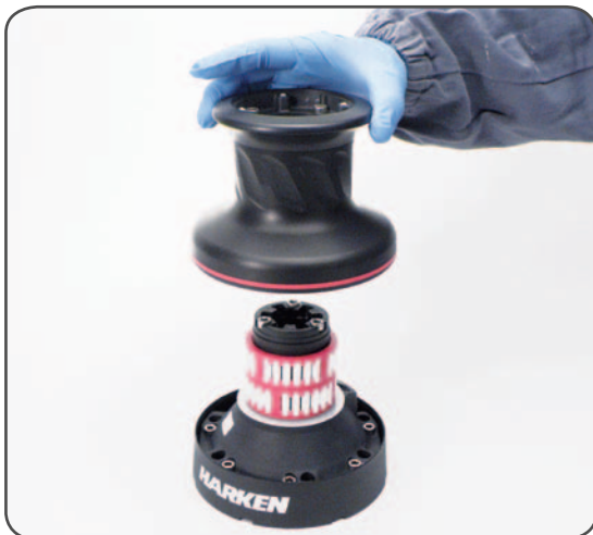
3. Lift off the drum n°22
