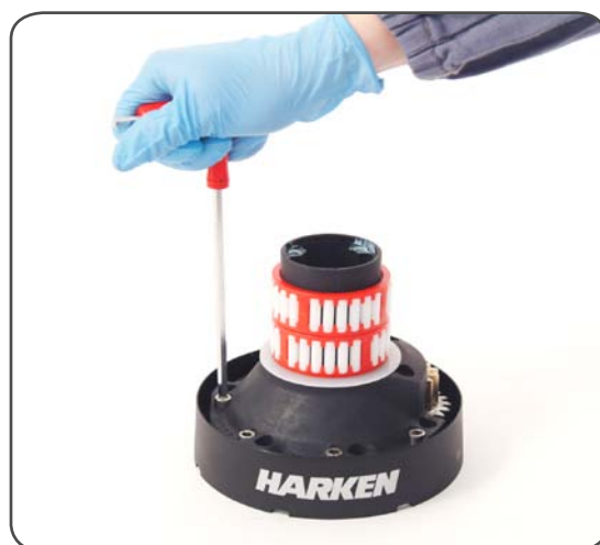
5. Remove the socket support n°21
