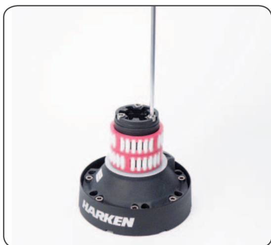
4. Completely unscrew the three screws n° 29
