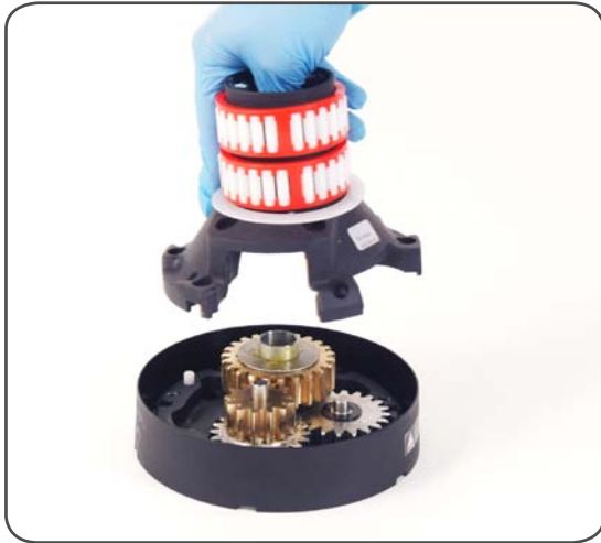
8. Remove the drum support n°15 Important: washer n°12 may remain inside the drum support!
