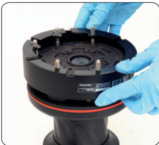
4. Reposition the skirt n°2 in its housing
