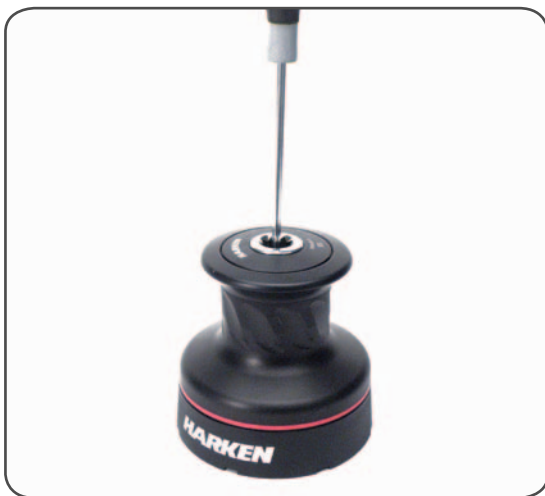
1. Unscrew the central screw ( \approx 2\text{Nm}/18\text{ in-lb} )
