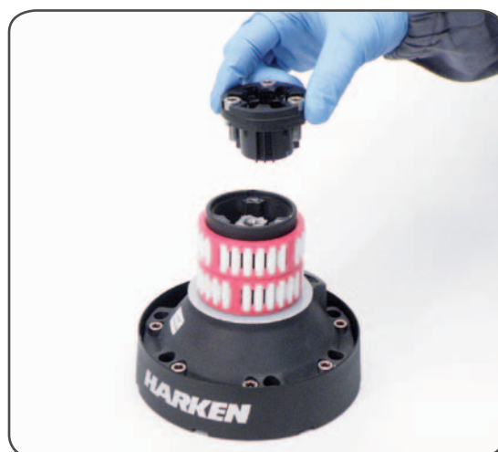
5. Remove the socket support n°21
