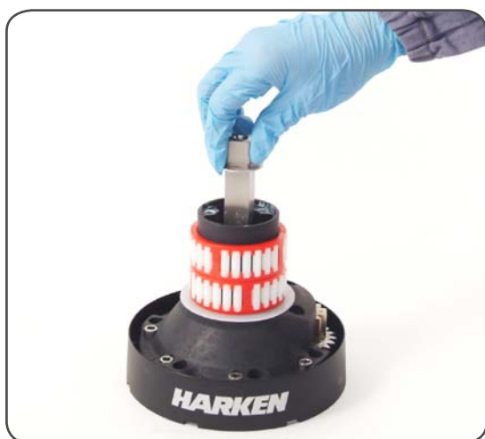
6. Slide out the central shaft n°19
