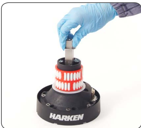
6. Slide out the central shaft n°19
