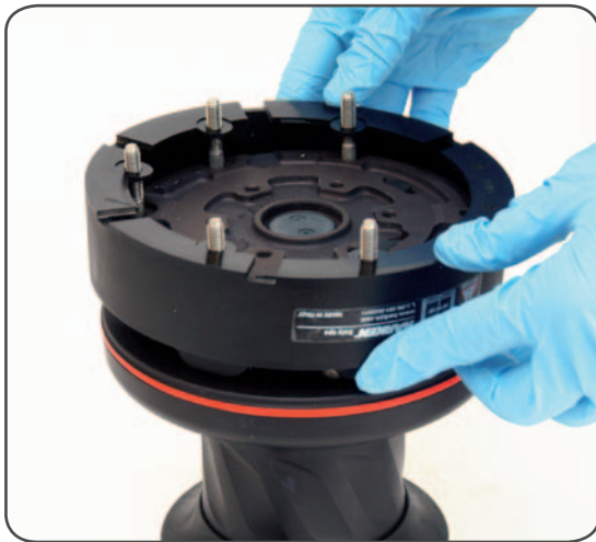
4. Reposition the skirt n°2 in its housing
