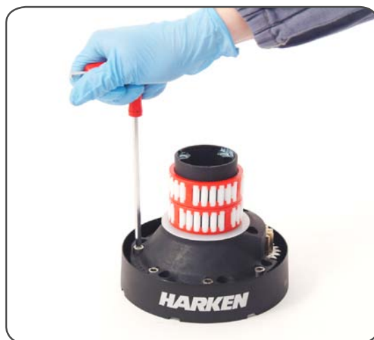
5. Remove the socket support n°21
