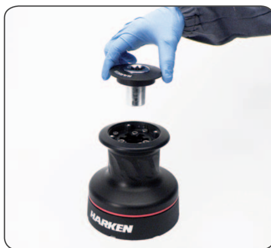
2. Slide off the hub n°30 and the cover n°27
