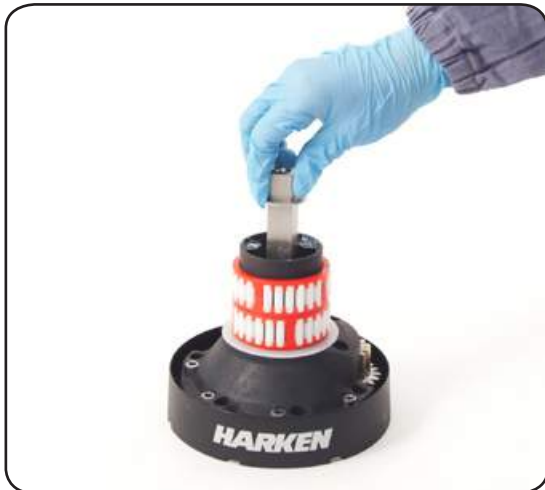
8. Slide out the central shaft n°19
