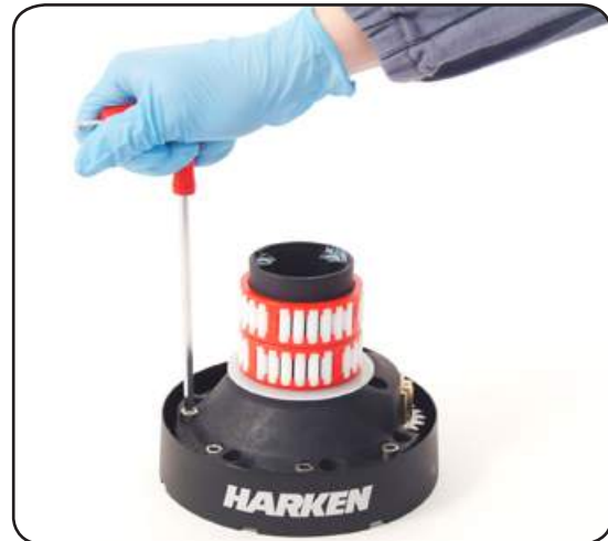
9. Unscrew the 6 hex screws n°16 ( \approx 8\text{Nm}/71\text{ in-lb} )
