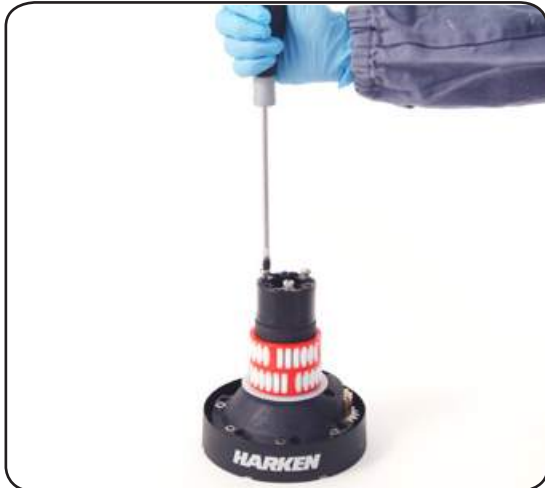
6. Completely unscrew the three screws n°27
