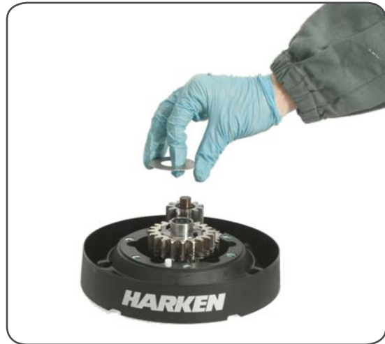
9. Remove the washer n°13 To facilitate the operation press the spring against the pawl with a blade.
