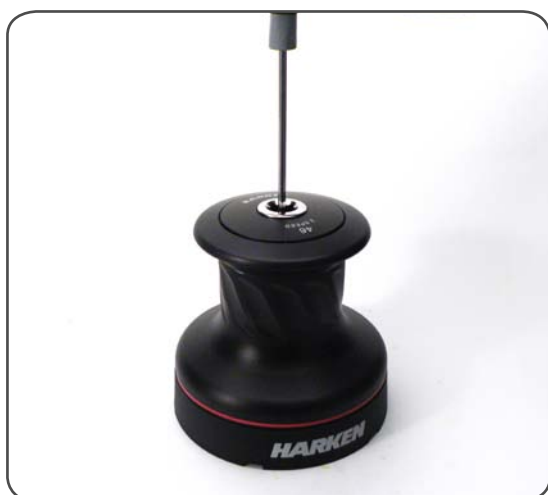
1. Unscrew the central screw ( \approx 2\text{Nm}/18\text{ in-lb} )
