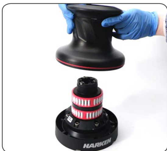
3. Lift off the drum n°23
