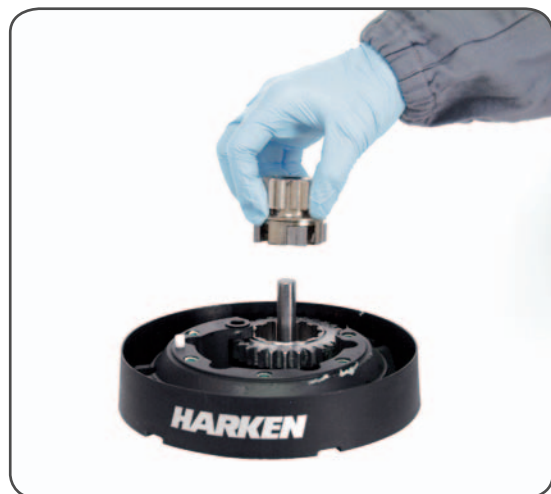
12. Remove the pinion n°11 To facilitate the operation press the spring against the pawl with a blade
