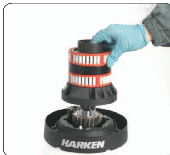
7. Remove the assy housing n°16 Important: washer n°13 may remain inside the drum support!
