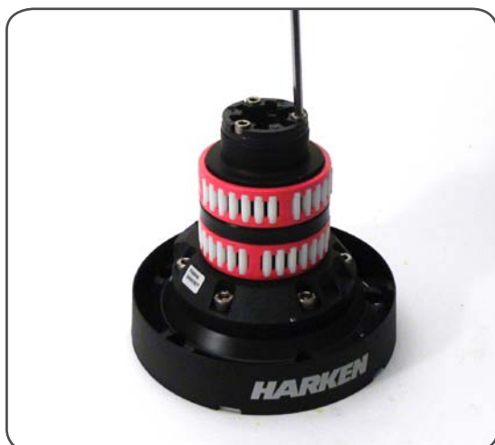
4. Completely unscrew the three screws n° 27 and remove the socket support n°22
