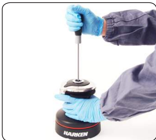
1. Unscrew the central screw ( \approx 2\text{Nm}/18\text{ in-lb} )
