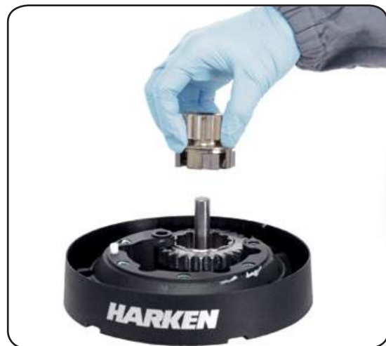
14. Remove the pinion n°11. To facilitate the operation press the spring against the pawl with a blade
