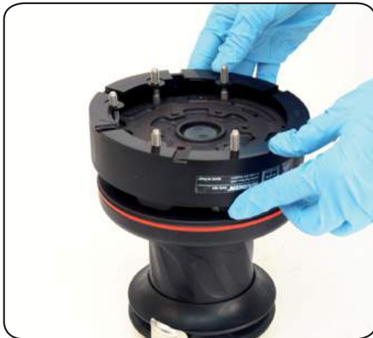
4. Reposition the skirt n°2 in its housing
