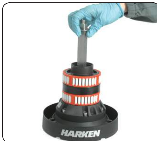
7. Slide out the central shaft n°21
