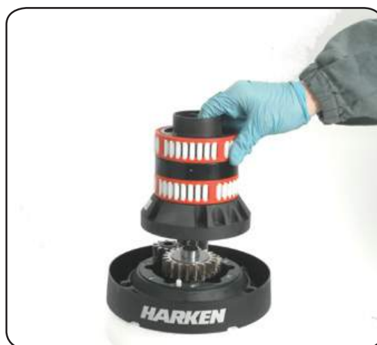
9. Remove the assy housing n°17 Important: washer n°14 may remain inside the drum support!
