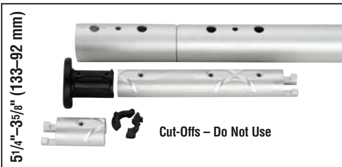
5 1 / 4 " - 3 5 / 8 " (133-92 mm) Do not use plastic bushing above top connector. Cut connector right at cross formed by glue dispersion channels. Use single foil screw in top foil only.
