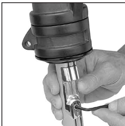
Loosen screw one revolution only .
