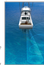
Without a fairing, the beam is angled improperly.
