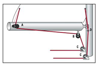
**Dual Line:** This dual-line system is common on boats 9 m (30') and larger. Position blocks so line pulls down and out to keep the sail flat and prevent lateral loads on the luff rope or luff sliders.
