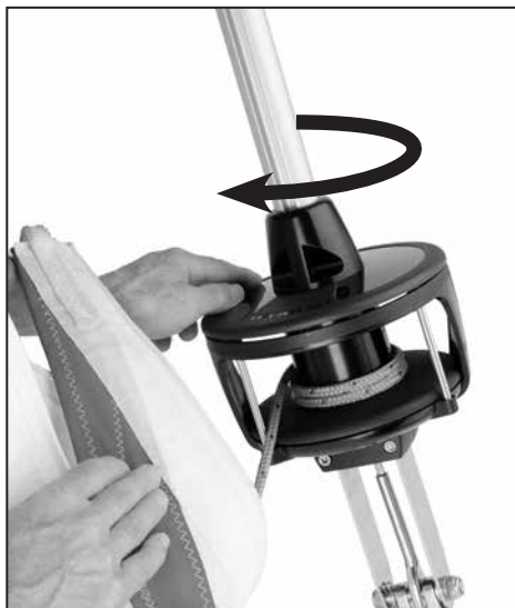
Sun cover on starboard side: wrap line by turning clockwise
