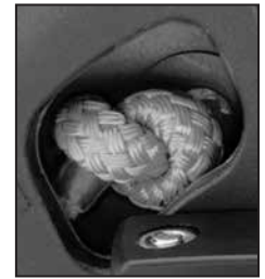
Tie a small overhand knot and pull it up tightly against spool. Spool must turn freely to furl and unfurl sail easily.
