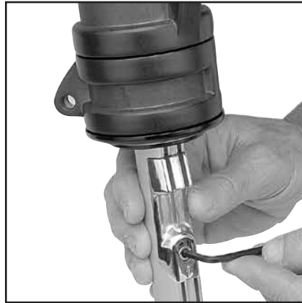
Loosen screw one revolution only .
