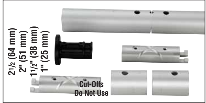
2 1/2"-1" (64-25 mm) Shorten top foil and adjoining full length foil so two screws are used to assemble joint instead of four. Do not use plastic bushings above top connector.
