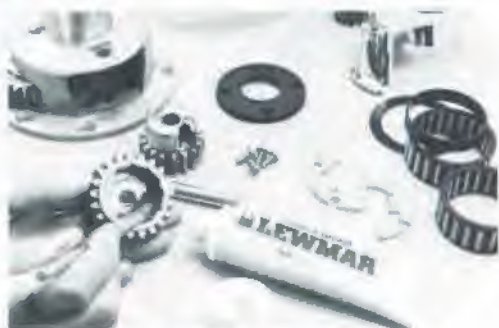
Lift out gear spindles, remove gears. Wash, clean and grease the gears.
