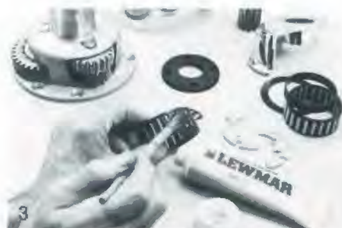
3 Remove stripper arm, drum. Release self tailing jaw assembly, clean and refit. Remove bearings and drum washer. Wash, clean and grease bearings.
