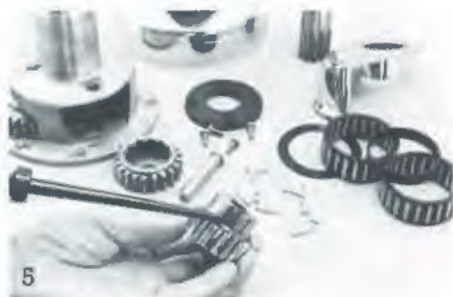
Lift out gear spindles, remove gears. Wash, clean and grease the gears.
