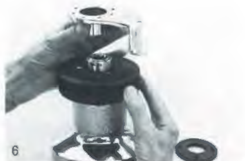
6 When reassembling take care that stripper arm is over stripper ring in jaw assembly. Reassemble winch in reverse sequence. Check for correct operation.
