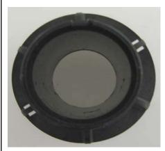
NOTE: The P17, B17, and SS557 (2" diameter) housings do not have a built-in valve. The valve sleeve (shown above) is separate from the housing. The installer slides the valve sleeve into the housing during installation.
