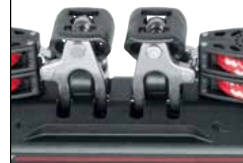
Toggles have a low pivot point to handle mainsheet loads up to 40 degrees from vertical, while allowing cars to roll freely.
