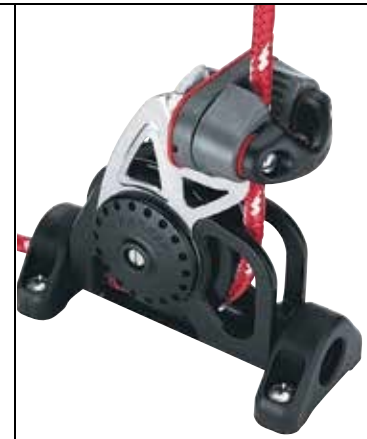
Block pivots around the line axis to keep line entry height low.
