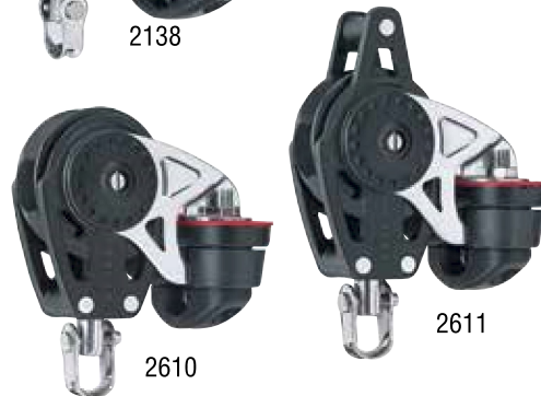
Switch locks shackle in front or side positions, or lets block swivel to keep line from twisting.
