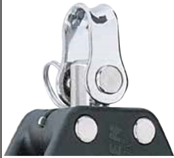
Switch locks shackle in front or side positions, or lets block swivel to keep line from twisting.
