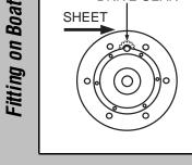
Position drive gear where sheet enters winch drum.
