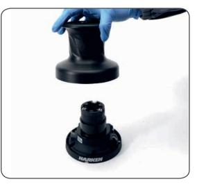
2. Lift off the drum n°13 with the socket n°17 and the washer n°20. Important: pay attenion to the pawls n°4 inside the plain top.
