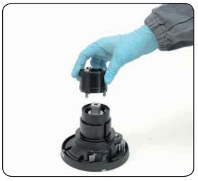
7. Remove the stripper arm support  $n^{\circ}12$  and slide out the bushing
