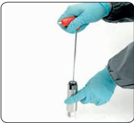
Unscrew the screw n°10 and remove the washer n°9 (%4Nm/35 in-lb)
