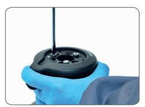
3. Unscrew the three screws n°16 (<sup>3</sup>√4Nm/35 in-lb)
