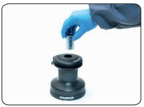
2. Slide off the socket  $n^{\circ}18$  and the cover  $n^{\circ}17$
