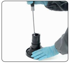
6. Completely unscrew the three screws n°16
