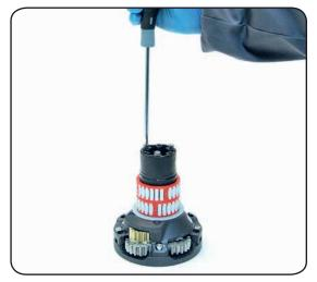
6. Completely unscrew the three screws n° 25
