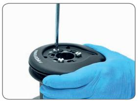
3. Unscrew the three screws n°25 (<sup>3</sup>√4Nm/35 in-lb)
