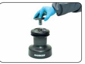
2. Slide off the assy socket  $n^\circ 27$  and the cover  $n^\circ 26$
