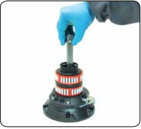
7. Slide out the central shaft  $n^\circ 19$
