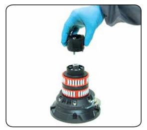
6. Completely unscrew the three screws  $n^\circ\,26$  and remove the stripper arm support  $n^\circ21$
