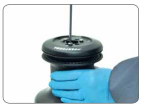
3. Unscrew the three screws n°25 (∛4Nm/35 in-lb)
