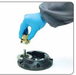
14. Remove the pinion  $n^{\circ}10$ .
