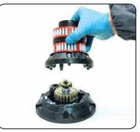
9. Remove the assy housing n°15 Important: washer n°13 may remain inside the drum support!
