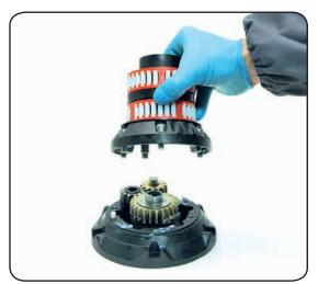
7. Remove the assy housing n°16. Important: washer n°13 may remain inside the drum support and the washer n°30 must be replaced in the correct position.
