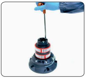
4. Completely unscrew the three screws n° 26 and remove the sochet support
