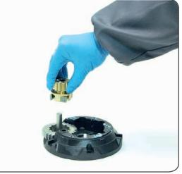
12. Remove the pinion  $n^{\circ}10$ .
