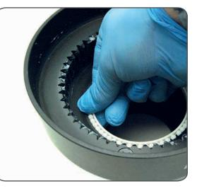
Once the winch is completely disassembled, clean the parts: use a basin of diesel oil to soak metal components and rinse plastic parts in fresh water. Once you have done this, dry the parts with cloths that do not leave residue.
