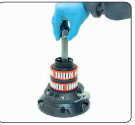
5. Slide out the central shaft  $n^\circ 20$
