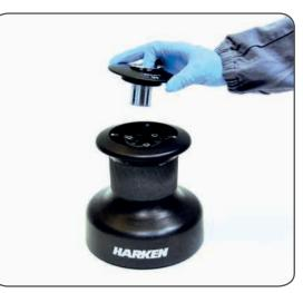
2. Slide off the hub  $n^\circ 29$  and the cover  $n^\circ 27$  and the washer  $n^\circ 31$
