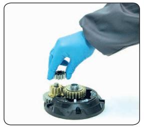
10. Remove gear  $n^{\circ}15$
