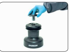
2. Slide off the assy socket  $n^\circ 29$  and the cover  $n^\circ 28$
