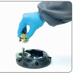
14. Remove the pinion  $n^{\circ}10$ .
