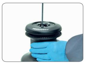
3. Unscrew the three screws n°27 (∛4Nm/35 in-lb)
