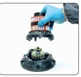
9. Remove the assy housing n°16 Important: washer n°13 may remain inside the drum support!
