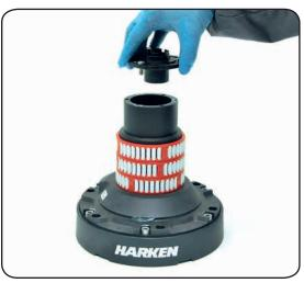
7. Remove the stripper arm housing n°21
