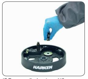
17. Remove roller bearings  $n^{\circ}12$ .
