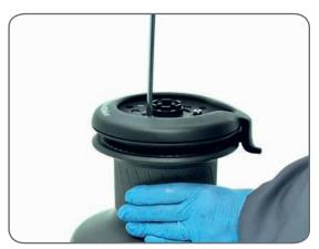
3. Unscrew the three screws n°26 (~4Nm/35 in-lb)
