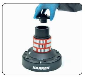
7. Remove the stripper arm housing n°21
