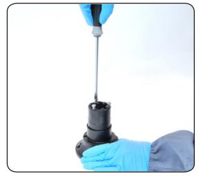
6. Completely unscrew the three screws n°17
