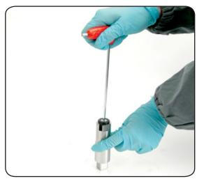
Unscrew the screw n°13 and remove the washer n°12 (~4Nm/35 in-lb)
