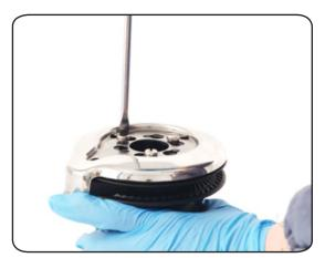
3. Unscrew the three screws n°17 (~4Nm/35 in-lb)
