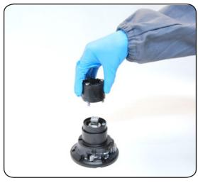
7. Remove the self-tailing arm support  $n^{\circ}2$  and slide out the bushing
