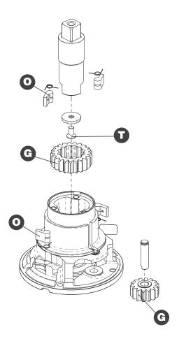
1. Apply Harken® grease on assy socket screw - 2. Apply Harken® grease on drum gear
