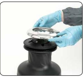
4. Remove the self-tailing arm n°27 by rotating and lifting it.
