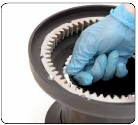
Once the winch is completely disassembled, clean the parts: use a basin of diesel oil to soak metal components and rinse plastic parts in fresh water. Once you have done this, dry the parts with cloths that do not leave residue.
