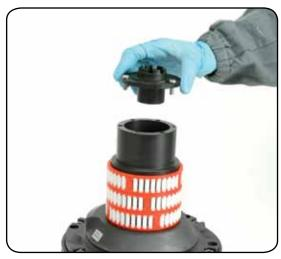
7. Remove the stripper arm housing n°21
