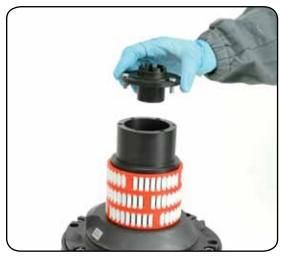
7. Remove the stripper arm housing n°21
