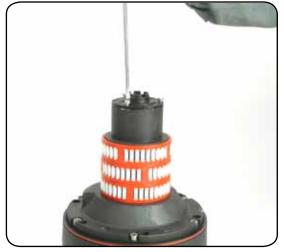
6. Completely unscrew the three screws n° 28
