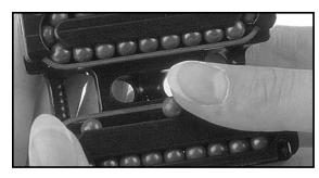
Position car on edge with retaining clip in place. Gently push one (1) ball at a time into car from center of clip. Allow balls to roll into return race and insert remaining balls. **Do not overfill car!**
