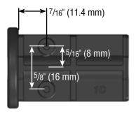
Drill two 1/8" (3 mm) holes in foil for self-tapping screws.
