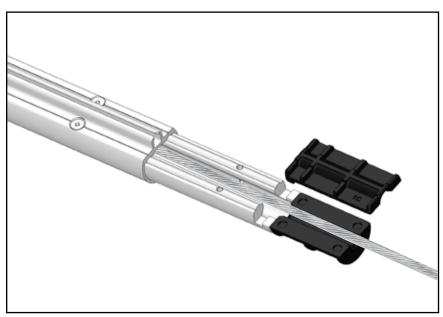
Put a drop of red Loctite® into screw holes.
