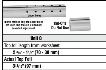
**Do not cut top foil** to length from worksheet. Cut top foil to  $3^{13}/16^{"}$  (97 mm) and shorten trim cap by  $3/4^{"}$  (19 mm) as shown at left. Shorten bottom foil per chart below. Foil will be clamped in **upper holes**.
