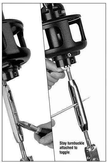
Lift foils so top is 3/8" (10 mm) below upper terminal. Use Tef-Gel on foil clamp screws when you replace them.
