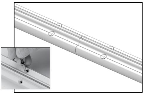
Slide halyard swivel onto foil. **IMPORTANT!** Make sure up-arrow is up.
