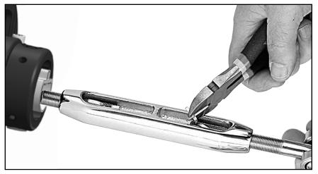
Slide lower drum assembly over turnbuckle and attach using long crosspin.
