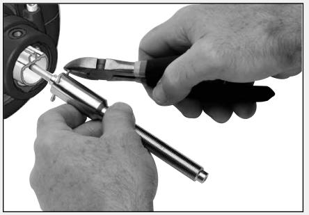
Assemble turnbuckle and attach Harken toggle.
