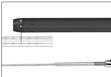
**Note:** Position top foil so that with top cap the foil will ride 3/8" (10 mm) below terminal. If wire fitting at top of stay is swage, foil must ride just below shoulder of swage. Mark cut line on foil. Wrap tape around foil as a guide so cut is straight.
