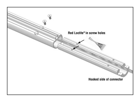
Use a hex key wrench to securely tighten screws.
