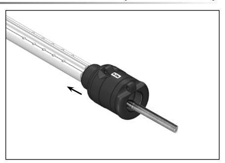
Slide drum assembly onto foil.
