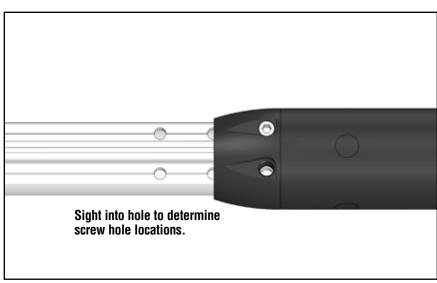
Slide halyard swivel above feeder. Place feeder tabs in position. Use a drop of 833 Blue Loctite® in screw holes. Use hex key wrench to secure.
