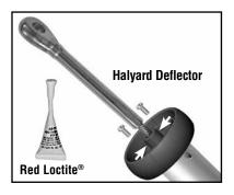
Put a drop of red Loctite<sup>®</sup> in screw holes. Place connector on wire with hooked side up.
