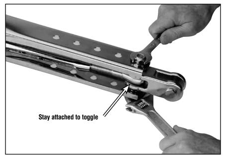
If stay length is set, use side cutters or needle-nose pliers to bend cotter pin to secure turnbuckle.
