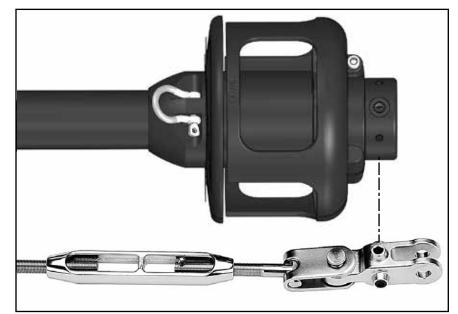
Line up bottom foil so foil clamp is just above or below center of notches in bottom foil.
