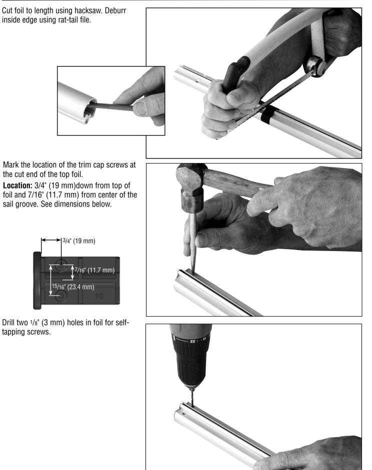
The following instructions cover installing foils on stay starting from the bottom. Foils slide over a swage stud fitting or wire end where a Norseman-/Sta-Lok®-type stud is used after foil assembly.
