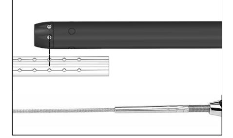
**Note:** Position top foil so that with top cap the foil will ride 5/8" (16 mm) below terminal. If wire fitting at top of stay is swage, foil must ride just below shoulder of swage. Mark cut line on foil. Wrap tape around foil as a guide so cut is straight.
