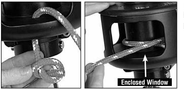
Run line through enclosed window in guard and into hole in bottom plate of spool. Tie a small overhand knot and pull it up under drum assembly.
