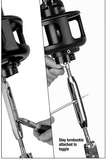
Lift foils so top is 5/8" (16 mm) below upper terminal. Use Tef Gel on foil clamp screws when you replace them.
