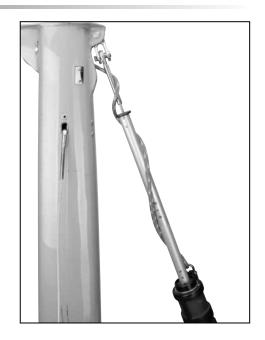
WARNING! Do not go aloft on boat's halyards if there has been a halyard wrap. Do not use boat. Damage to halyard, headstay, stay terminals, or connections as a result of a halyard wrap may cause these parts to break suddenly causing mast to fall down while person is aloft. Sailing or motoring with boat after a wrap can result in the headstay breaking and mast falling down. Before using boat, have a professional rigger inspect and replace parts as necessary using following methods.
