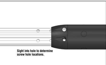
Slide halyard swivel above feeder. Place feeder tabs in position. Use a drop of 833 Blue Loctite<sup>®</sup> in screw holes. Use hex key wrench to secure.
