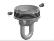
IMPORTANT! - Secure the torsion cable to the head swivel first. Wait to cut the torsion cable to length until you can check the length by dry fitting into the assembled drive unit with tack swivel and threaded adapter in place.
