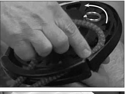
Rotate the drive sheave as you press the line into position around the drive sheave. Load the final part by pulling the line from outside the drive unit.
