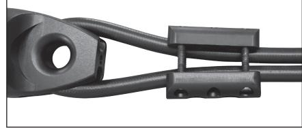
4. Push the clamp assembly toward the thimble. Squeeze the torsion cable at the thimble. Position clamp about 10 mm (3/8") from the thimble as shown. Make the tail of the cable about 90 mm (3.5") beyond the clamp.
