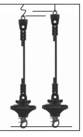
Note: When using an A2 sail, it is important to maximize the cable length so the sail can be at full hoist. The best way to achieve the maximum is to add to the cable length, then adjust the cable length after sailing. When sailing, tension the halyard only enough to pull slack out of the Reflex torsion cable.
