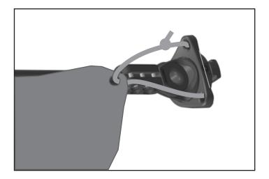
Load the Reflex tack terminal into the T-slot on the lower drive unit. Attach the unit to the bow sprit or a fixed point on the bow ahead of the stay. Attach halyard to head swivel and check halyard and sheet leads. Hoist and trim spinnaker.
