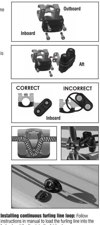
instructions in manual to load the furling line into the furler. Load the line into the fairleads by bending into the openings. Push the line into place.
