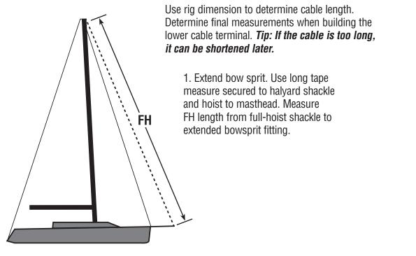
2. The required untensioned cable length roughly equals the FH length. The length may seem too short as illustrated by the "straightened" cable beyond the FH length as seen on the diagram. See ends labeled STR at right. The STR length is gained back by stretch over the full torsion cable when the system is tensioned when hoisting the spinnaker. Note: The amount of halyard tension to furl the sail using the Reflex torsion cable is moderate compared to other systems.
