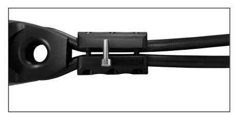
6. Continue to tighten the four (4) corner fasteners until the gap between the clamp halves is around 5 mm (3/16"). Now tighten the two center fasteners until snug.
