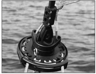
The furling action when furling an asymmetric spinnaker and tack swivel terminal is top-to-bottom; furling starts at the sail head and moves downward.
