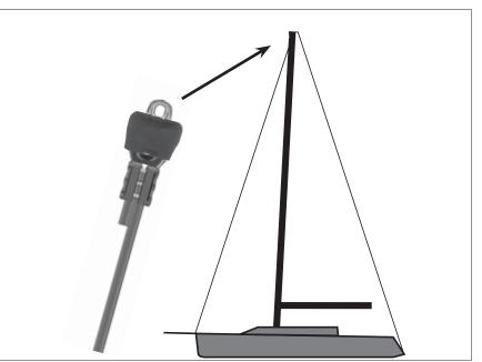
Install the tack swivel terminal on the drive unit by pulling the locking spring pin and slipping the T-foot of the terminal into the T-slot in the drive unit. Make sure the snap shackle threaded adapter or alternate adapter is assembled to secure the unit to the boat.
