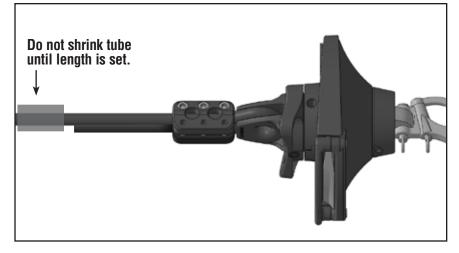
**8. Checking the length:** Attach the drive unit to the bow fitting or pole. Hoist the cable without sail to check the length. Use the halyard winch to tension the halyard enough to straighten the cable.
