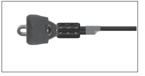
10. If assembling away from the boat, lay cable out straight. Install tack terminal and snap shackle adapter on drive unit. **Note:** See following pages for preferred method of determining length at boat.
