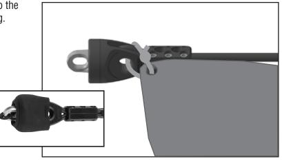
**Asymmetric spinnaker:** Secure tack of sail using soft-attach long shackle. Make length adjustable for adjustment when sail is finally fitted.
