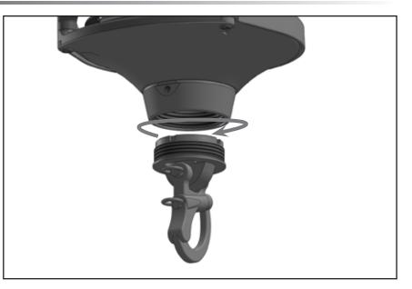
Back the adapter out no more than one (1) rotation until the set screw holes line up with the recesses at the top of the threaded adapter. Sight into one of the set screw holes to confirm alignment.
