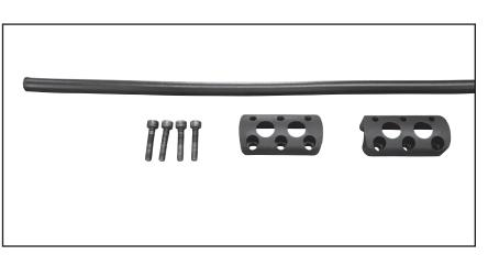
Cut heat-shrink tubing to half length and slide the half onto the cable. Assemble the clamp halves near the cable end using four (4) longer screws threaded into the corner holes. Turn several turns as shown and leave enough space to load the cable end.
